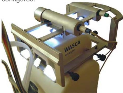
DSA is designed as an easy to use high precision optomechanical plug-on to the aberrometer cover and includes additional configurable driving electronics and sophisticated application software. The installation of the DSA package does not require extended technical changes of your aberrometer system but simply adds additional functionality. This functionality extends the capabilities of your aberrometer system and allows you to go beyond today's limitations!
